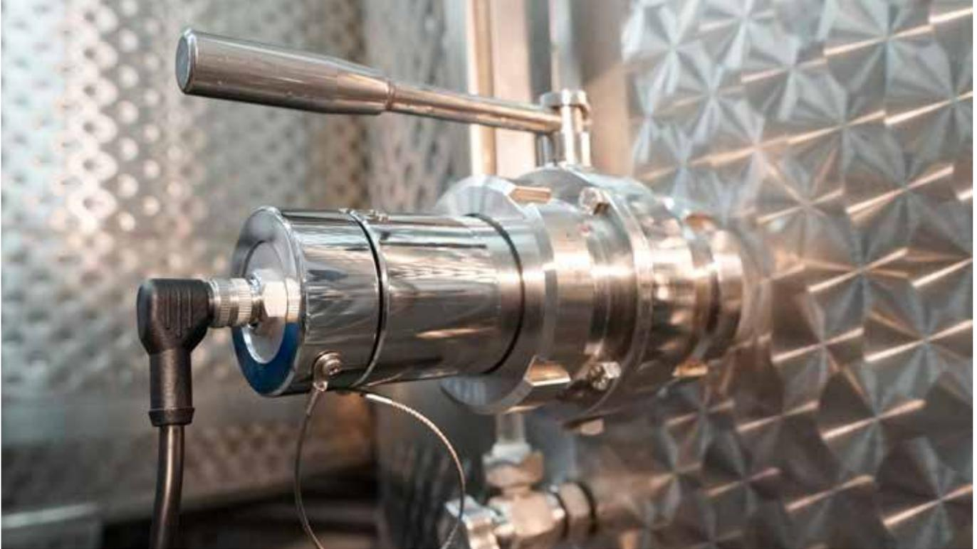
VinPilot® Brix digital refractometer inserted through a DN 50 ball valve.
